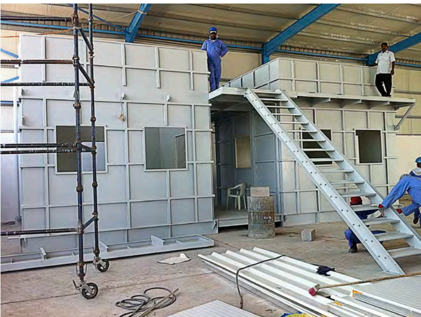
Diving tanks for Wet Welding and NDT
