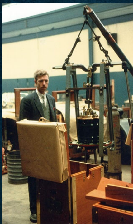
FINAL ASSEMBLY STAGE OF A PUMP DUE FOR SHALLOW WATER DIVING WORK IN AFRICA
