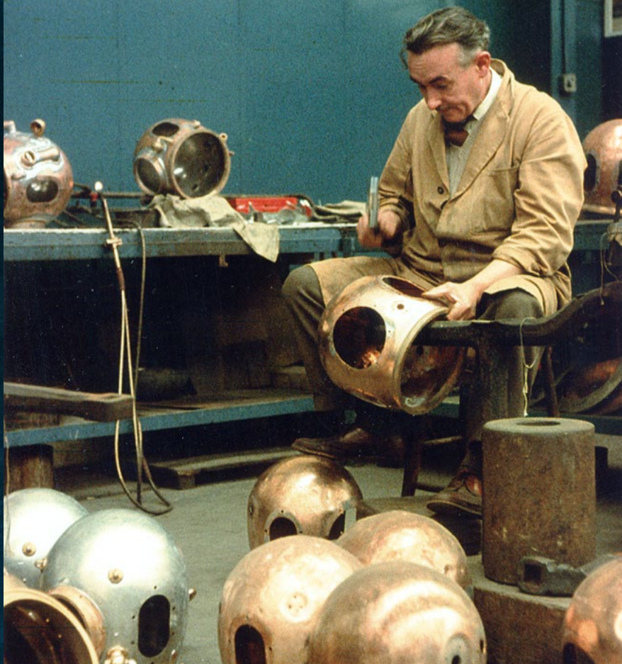
THE COPPERSMITH AT HIS BENCH, REFINING THE BASIC METAL SHAPE TO ACCEPT VALVES, PORTHOLE AND VARIOUS OTHER FITTINGS. IT WAS MORE ARTISTRY THAN INDUSTRY.
