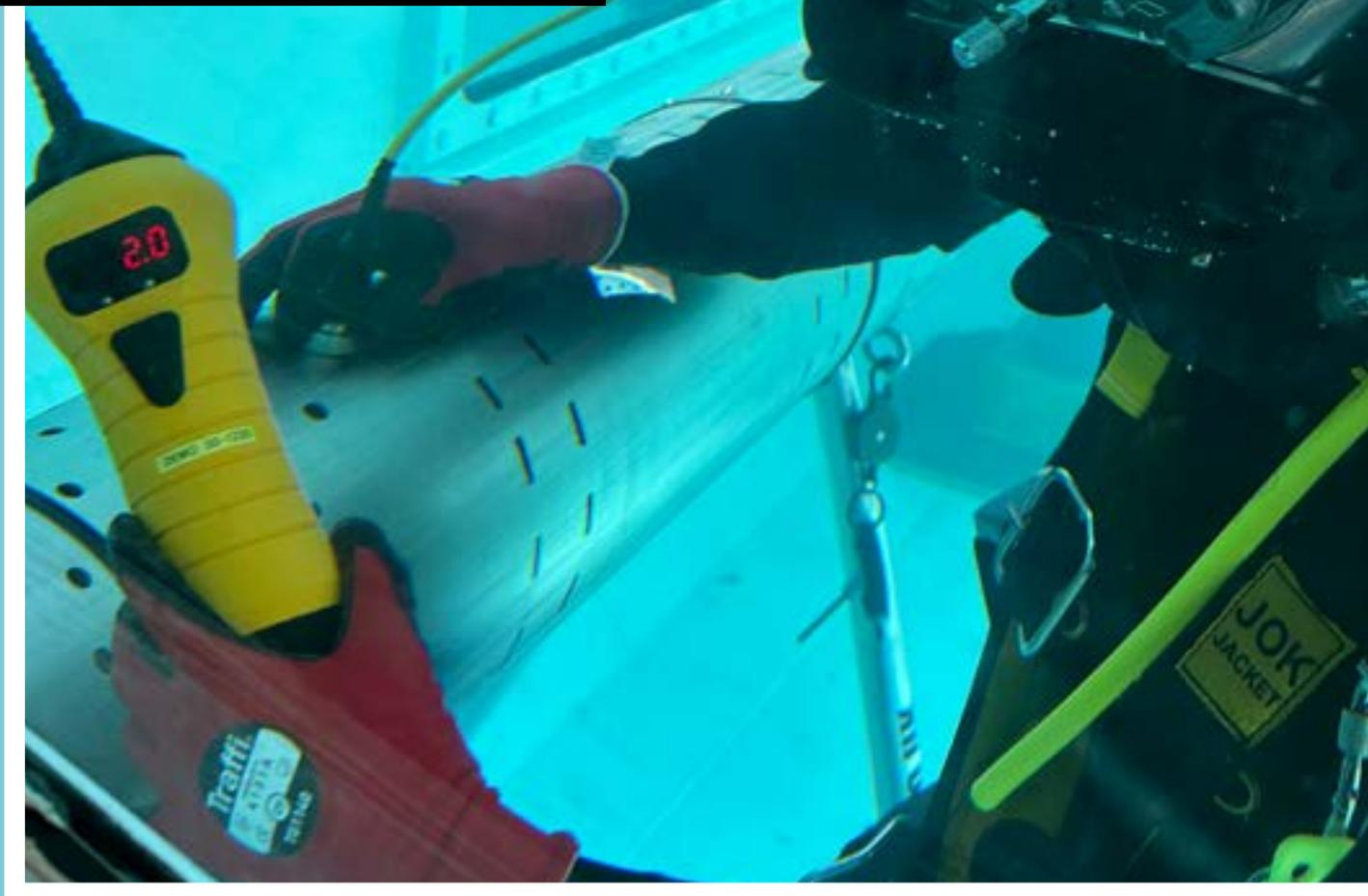
**Tritex NDT have for many years been manufacturing ultrasonic thickness gauges and are now established as one of the leading companies offering multiple echo gauges. Multiple echo technology means that thickness measurements can be taken through 6mm thick coatings, only the metal substrate is measured. This technology is therefore ideal for use with an underwater thickness gauge to save both time and money.**
