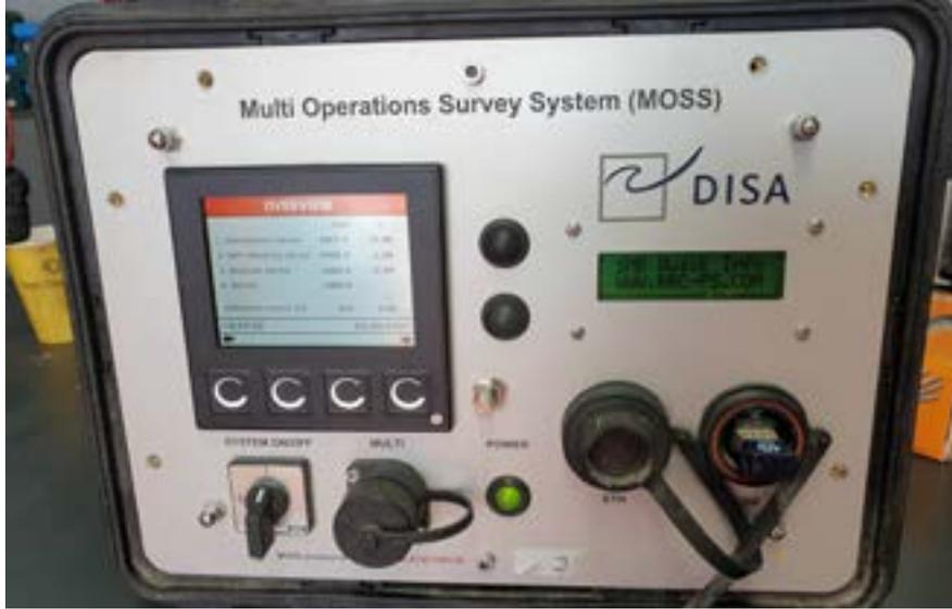
Additional to the improved accuracy on the measured data also a practical improvement was the cabling. The first prototype had a separate cable to the sensor at the diver. As the 4-core video line is often not used by the diver it was made possible that the sensor can be connected to this connector and the data is retrieved again on the surface and connected to the logger unit. So no additional cable is needed anymore.
