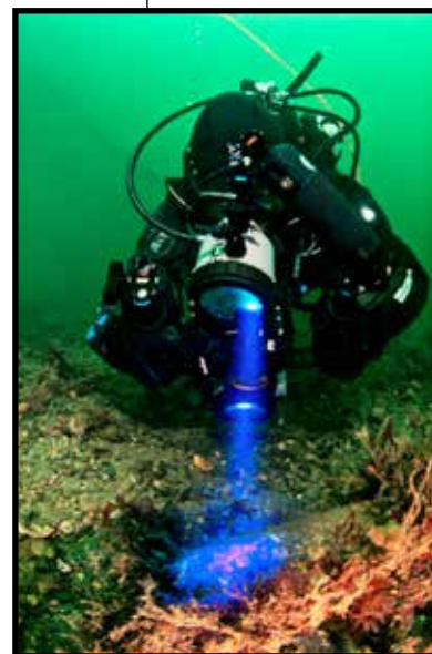
NFSD divers evaluating the underwater application of LiDAR (Light Detection And Ranging) and fluorometric photography
