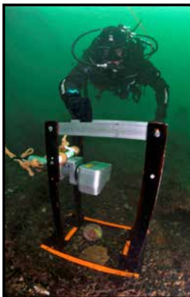
NFSD divers evaluating the underwater application of LiDAR (Light Detection And Ranging) and fluorometric photography
