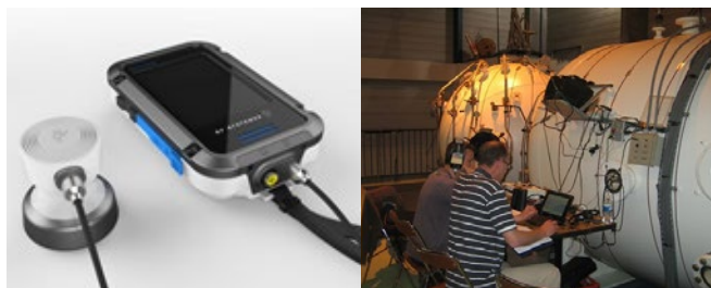
Azoth Systems Precordial Doppler prototype in 2013 & Tests during the NATO Submarine Rescue System decompression table validation
