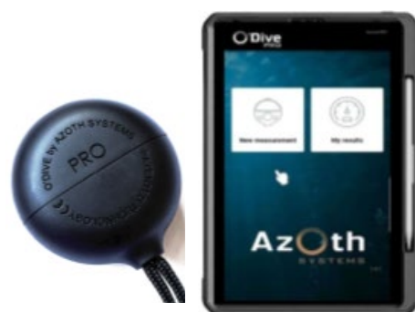
Subclavian Doppler sensor assisted with software for a self-monitoring by divers themselves
