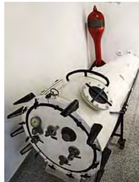
A hyperbaric chamber for one person only, used to transport injured divers
