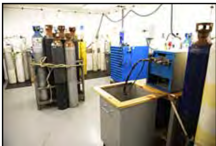
The school has a blending station for oxygen and helium from which they make all the gasses as required. Gases can be produced and mixed for specific depths.
